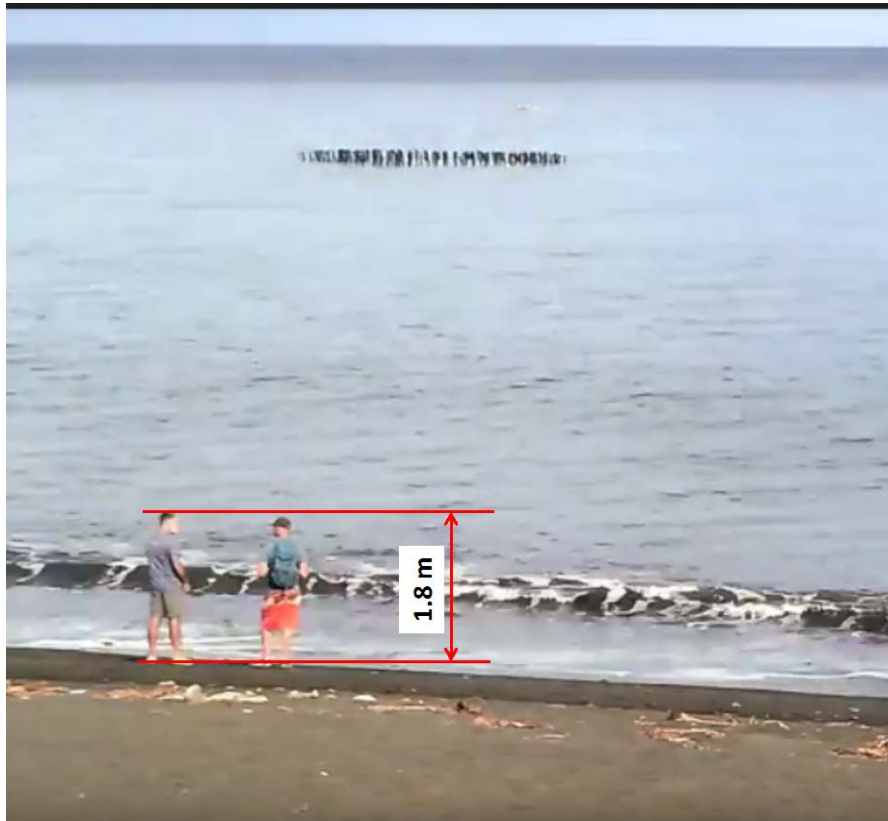
This portion of the video clip, when the 1.8m reference height is in line with the SSB made it possible to calibrate pixel scale at the shoreline
