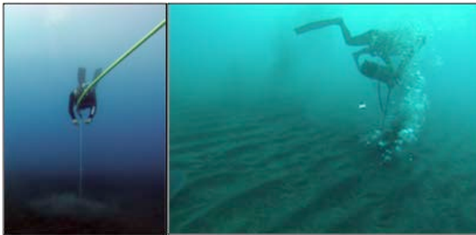
Figure 4: Underwater probing of the sea-floor, by using a waterjetprobe on the left and airjetprobe on the right, for assessing the sand depth and sea-substrate characteristics (Diver: Michael Rutzen; Photographer: Sara Andreotti)
