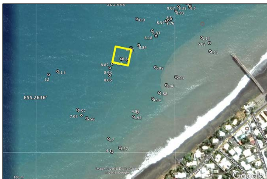
Figure 5: The proposed location identified for the exclusion test at Saint-Paul. The preferred location is based on the depth, the characteristics of the sea-floor and the estimated wave action. (Base image: Google Earth™)
