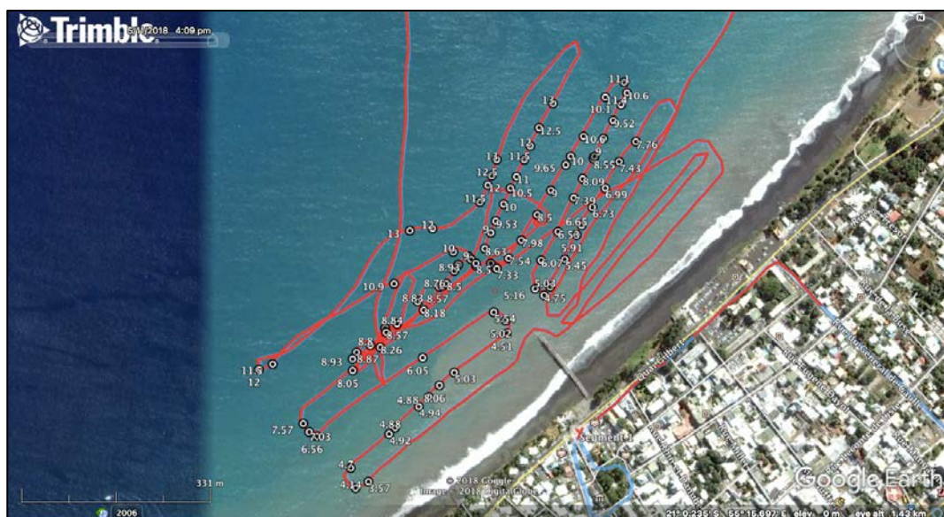
Figure 3: The water depth along transects in the selected area of deployment was surveyed by boat to identify an area at which the SSB Unit can be deployed to form the required shark exclusion area. (Base image: Google Earth™)
